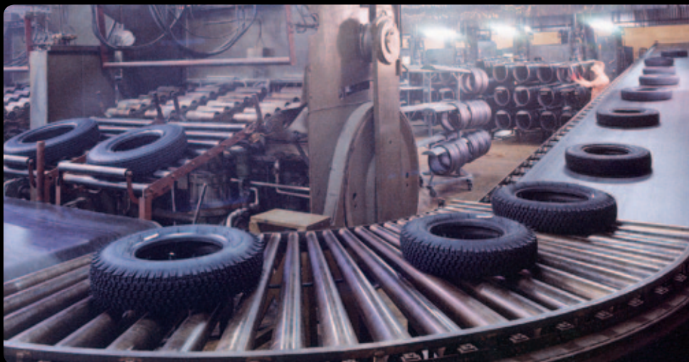
Fresh tyres are transported from curing moulds to the conveyor. The new tyre plant in the early 1970s. Photo: Pauli Lehtioksa.
